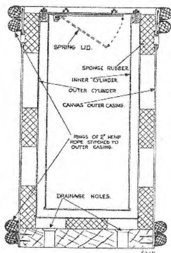
Fig. 1a. First model of new bucket.
