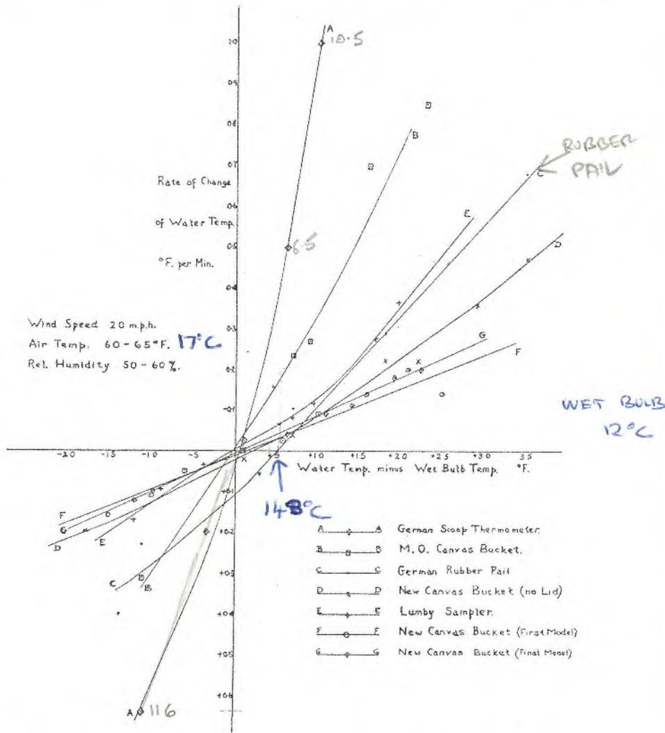
Fig. 2. Rate of change of water temperature in bucket as a function of the difference between the water temperature and the wet bulb temperature.
