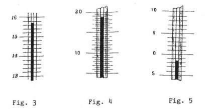
Positions of the column of mercury against the different thermometer scales
