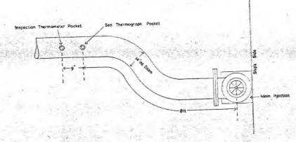
Fig. 2 Diagram showing the position of the thermometer in the engine-room intake pipe.
