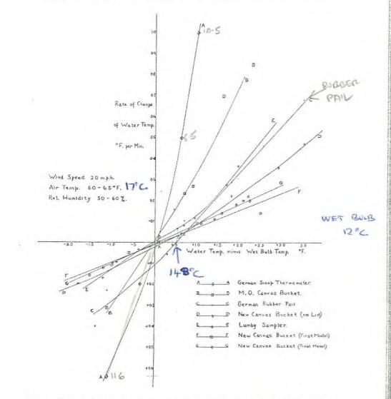
Fig. 2. Rate of change of water temperature in bucket as a function of the difference between the water temperature and the wet bulb temperature. 109
