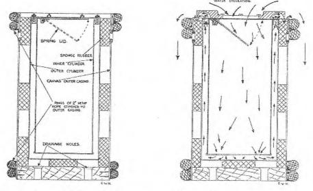
Fig. 1a. First model of new bucket.
